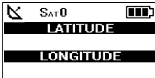
Figure 10 : GPS screen (No synchronisation)
